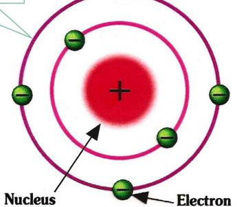
Using the extra energy from the photons, the electron then moves off of the valance band and is free to be used for electricity.
